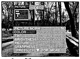
4. Press A or ♥ to select the desired Picture Adjustment (Color, Tint, Brightness, Picture, or Sharpness).
